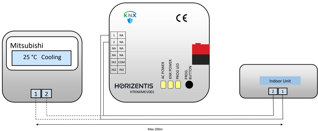
Wired remote controller must be in master mode if connected. In this case gateway must be set in slave mode from parameters.
