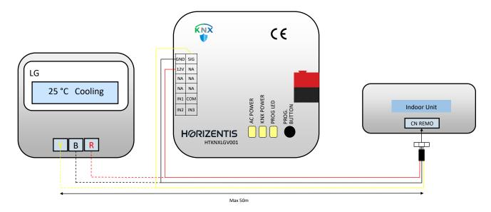
Wired remote controller must be in master mode if connected. In this case gateway must be set in slave mode from parameters. Connector cable supplied by Horizentis.
